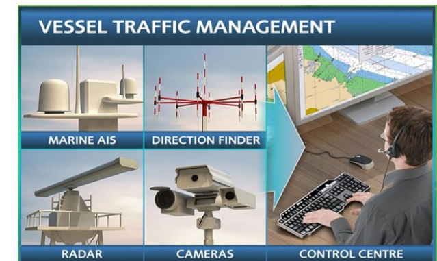
Vessel Traffic Management System (VTMS)
